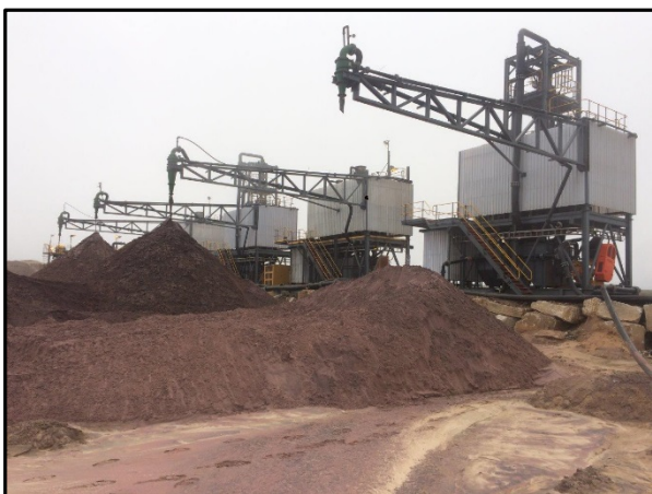
Two Primary Beach Concentrators and the two recently constructed and commissioned Tailing Scavenger Circuits. Depicting Heavy Mineral Concentrate production and stockpile.
