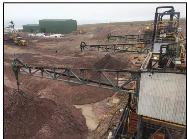
Two Primary Beach Concentrators and the two recently constructed and commissioned Tailing Scavenger Circuits. Depicting Heavy Mineral Concentrate production and stockpile.
